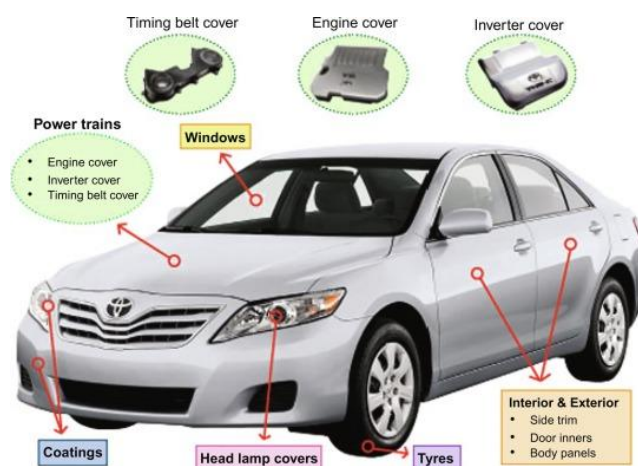
Figure 5. This image identifies various component of a car, made up of PNCs
